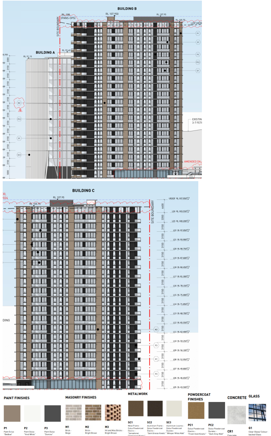
Figure 4 East Elevation showing materials and finishes
